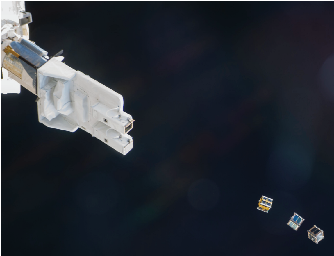
FIGURE 3.6 CubeSats being deployed from the International Space Station after being removed via the airlock in the Kibo module. SOURCE: Courtesy of NASA.
