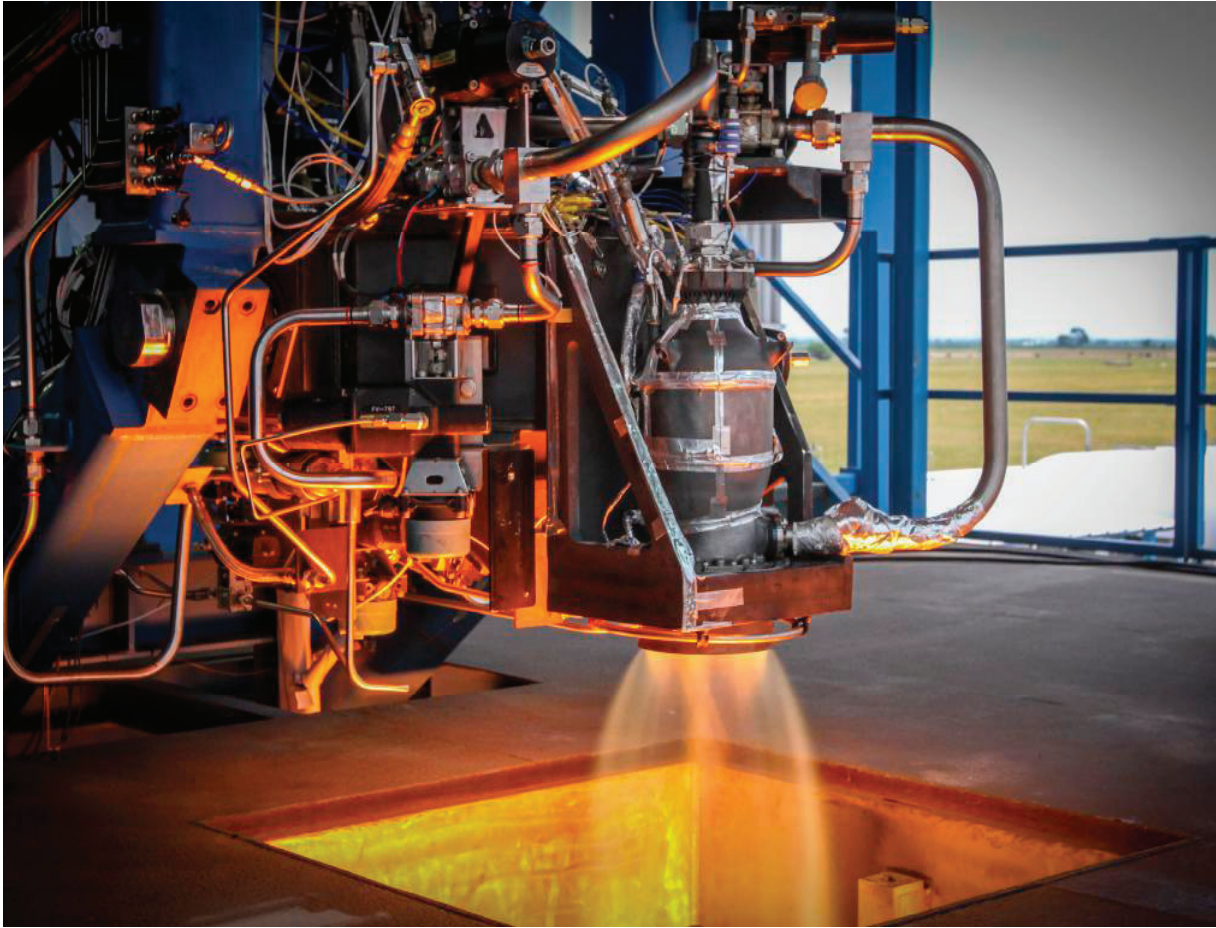
FIGURE 3.1 Test of a SuperDraco rocket engine at full power using an additively manufactured Inconel thrust chamber. SOURCE: Courtesy of SpaceX.
