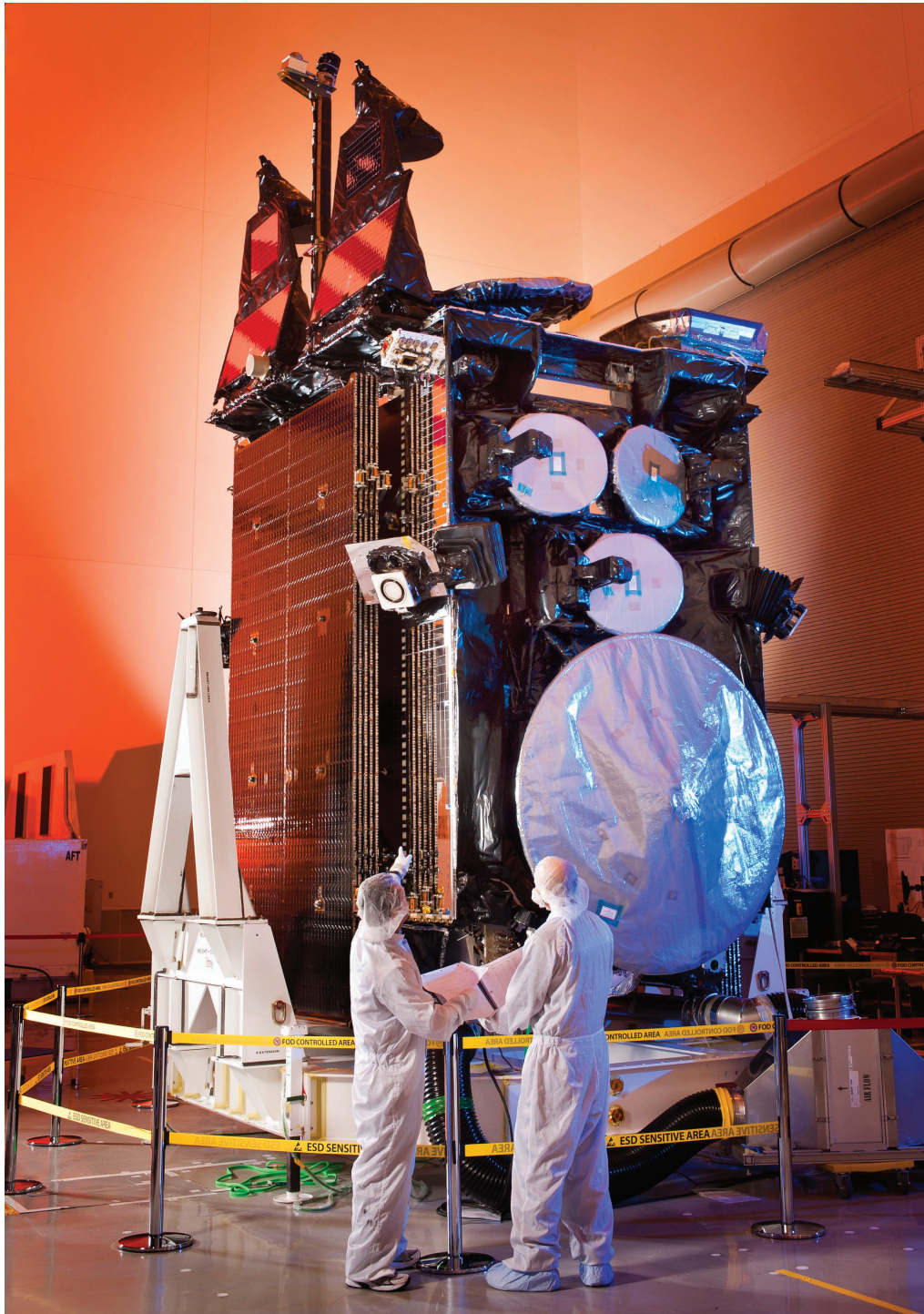
FIGURE 3.2 Lockheed Martin Advanced Extremely High Frequency communications satellite built for the Air Force. Many satellites constructed for operational military and civilian missions are large and complex. Although they may incorporate additively manufactured components, the next major challenge will be additively manufacturing major subsystems on the ground. SOURCE: Courtesy of Lockheed Martin Corporation.
