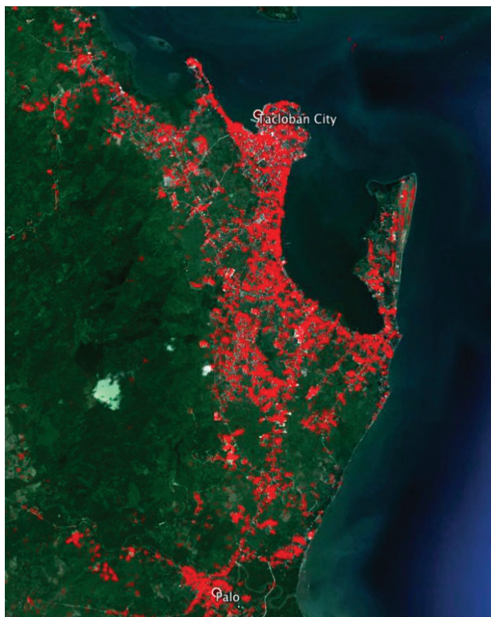
FIGURE 4.9 Interferometric “change map” derived from Italian Space Agency Cosmo-Skymed radar depicting damage done by Supertyphoon Haiyan in the Philippines, November 8, 2013. Areas in red reflect the heaviest damage to cities and towns in the storm’s path. SOURCE: ASI/NASA/JPL-Caltech. See NASA, “NASA Damage Map Helps in Typhoon Disaster Response,” November 13, 2013, http://www.nasa.gov/centers/jpl/news/typhoon20131113.html#.VZ15xvIvHbf .
