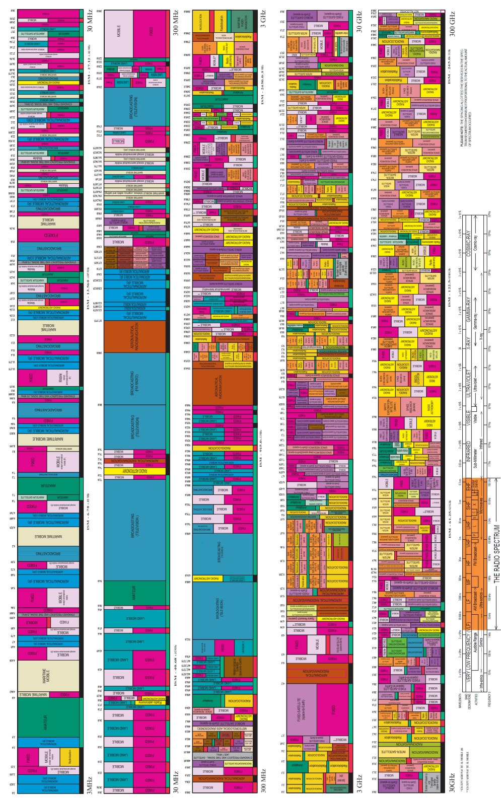
FIGURE C.2 U.S. radio spectrum allocations, from 3 MHz (top left) to 300 GHz (bottom right). Each colored block represents an allocation to one of 30 different services. Allocations to services most amenable to CubeSats are in orange (Earth exploration-satellite), dark brown (space operation), pale pink (space research), and light blue (amateur-satellite), but are generally too small to see at this scale. The largest blocks in this chart (blue) are for radio and television broadcasting. Note that this figure is presented as a visual example of the complicated nature of spectrum allocation. Full-resolution, specific details may be viewed on the NTIA's webpage. SOURCE: U.S. Department of Commerce, National Telecommunications and Information Administration, "United States Frequency Allocation Chart," https://www.ntia.doc.gov/page/2011/united-states-frequency-allocation-chart , accessed April 8, 2016.
