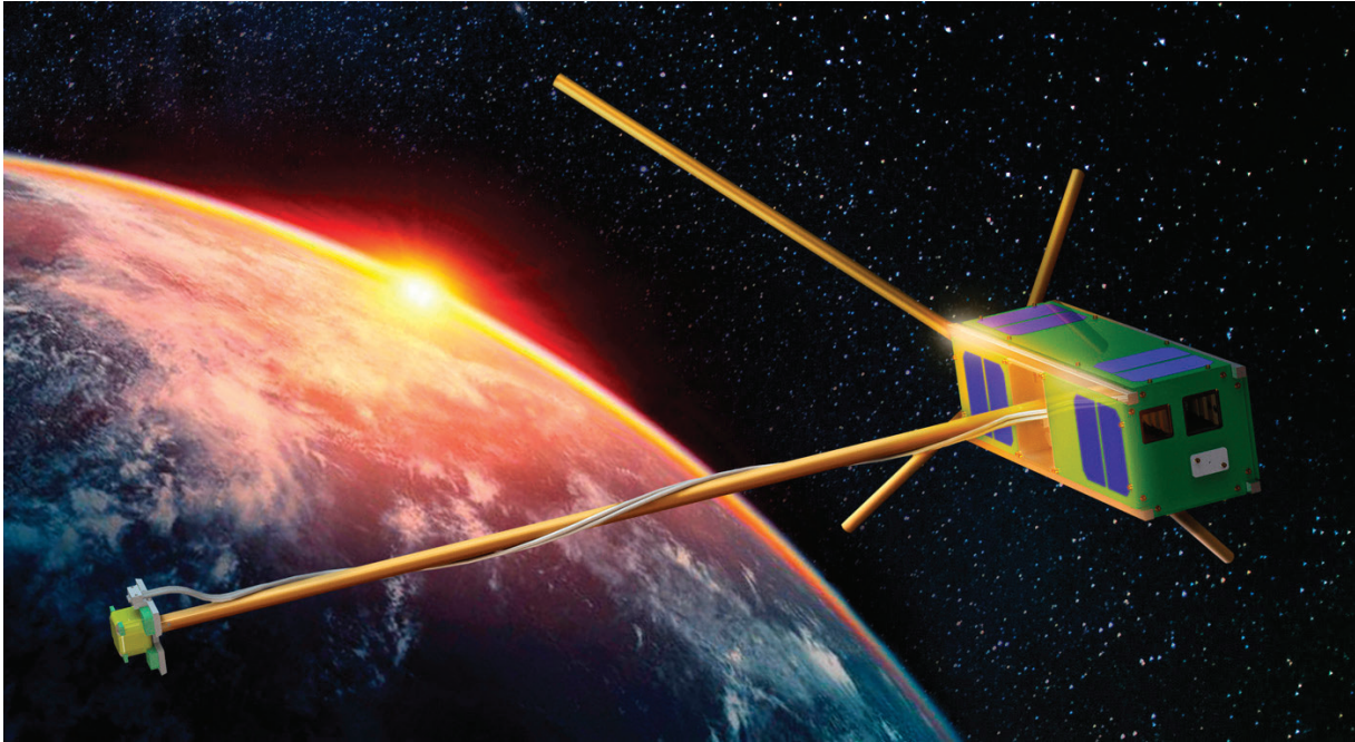
FIGURE 1.9 The ELFIN CubeSat was part of the University Nanosatellite Program. SOURCE: Courtesy of the University of California, Los Angeles.
