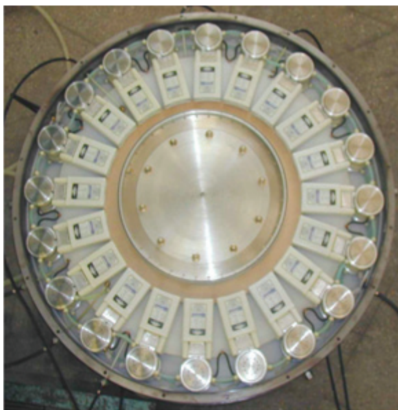
FIGURE 2-12 Top view of 20 units in parallel in an annular LTD cavity. SOURCE: Copied with permission of the first author from M.G. Mazarakis, W.E. Fowler, A.A. Kim, et al., 2009, High current, 0.5-MA, fast, 100-ns, linear transformer driver experiments, Physical Review Special Topics-Accelerators and Beams 12: 050401.
