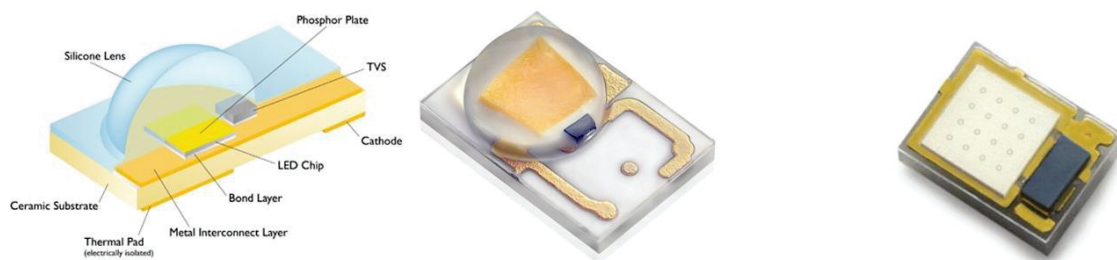
FIGURE 5.4 Thin-film flip-chip (TFFC) package. (a) Cross-section of TFFC. The package provides high luminance light source for directional applications. The contact/heat-sinking does not interfere with the light emission. The thin-film structure requires careful handling. (b) Domed and undomed light-emitting diode (LED). SOURCE: Images courtesy of Lumileds.
