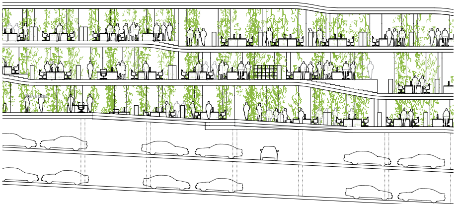
The floors of the buildings follow the natural topography of the site. The wings, some of them very long, are therefore divided into shorter, stepped sections
