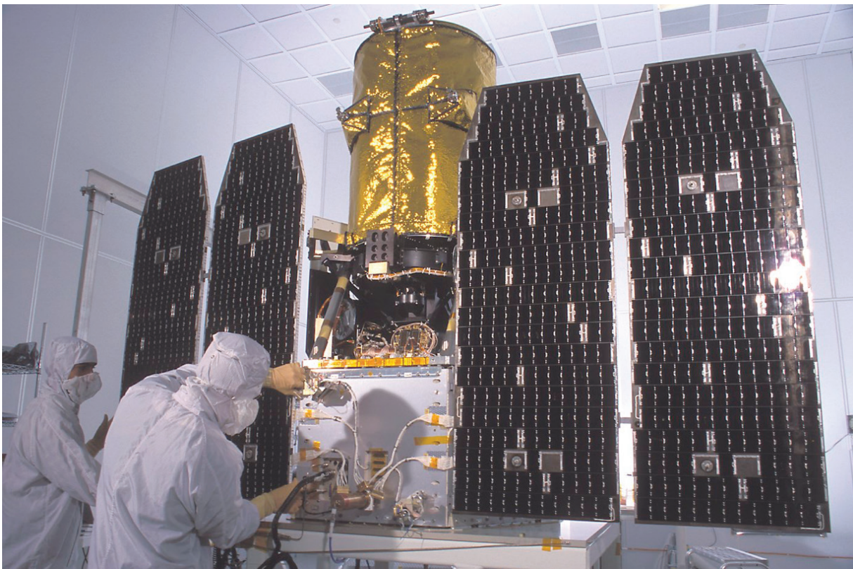
FIGURE 5.1 The Galaxy Evolution Explorer (GALEX) spacecraft during construction. SOURCE: GALEX Technical Documentation, “Chapter 1. Instrument Overview,” accessed June 27, 2016, http://www.galex.caltech.edu/researcher/techdoc-ch1.html ; courtesy of JPL/Caltech and the GALEX science team.
