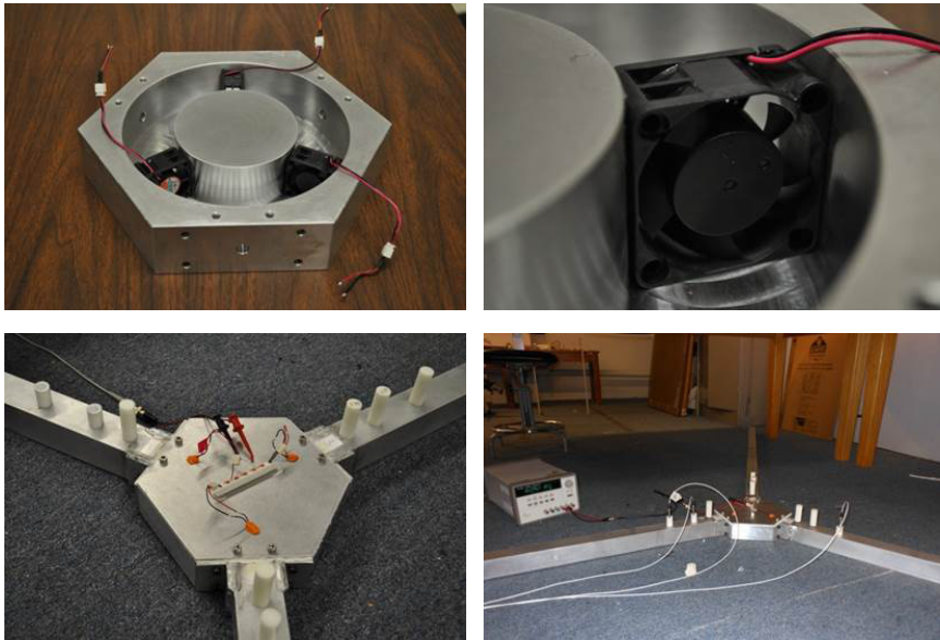
FIGURE 3 A table-top circulator that breaks the symmetry of acoustic wave travel in air. It is formed by a circularly symmetric cavity loaded with three CPU fans ( upper right ) that move air at a moderate velocity that is enough to break reciprocity and enable large isolation. The cavity is connected to three acoustic waveguides ( bottom left ) carrying sound signals. Adapted from Fleury et al. (2014c).
