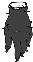
9. Cast bronze hand with core, chaplets, and clipped gate systems.
