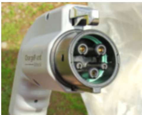
FIGURE 2-6 The SAE J1772 plug that connects all PEVs to AC level 1 and level 2 is an agreed-on universal standard for 120 V and 240 V ac charging. SOURCE: © Michael Hicks, licensed under Creative Commons 2.0 (CC-BY-2.0).
