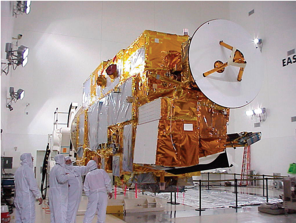
FIGURE 2.2 The Terra spacecraft undergoing final testing at Goddard Space Flight Center in the late 1990s. SOURCE: NASA.
