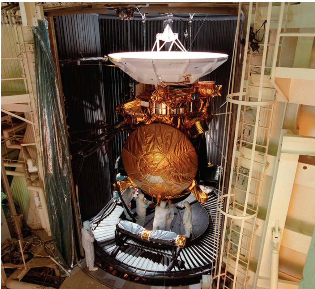
FIGURE 2.4 The Cassini-Huygens spacecraft during final integration and testing in the late 1990s. The Huygens atmospheric probe is the large gold disk at center. SOURCE: NASA.
