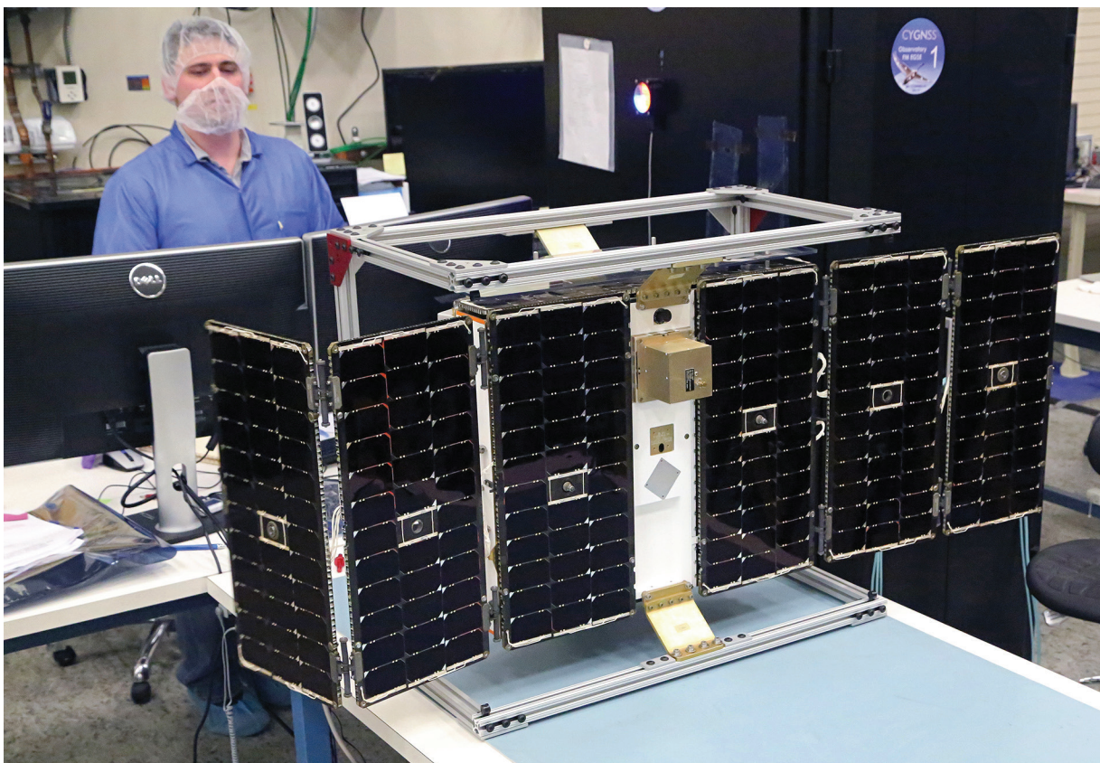
FIGURE 1.2 One of the CYGNSS (Cyclone Global Navigation Satellite System) spacecraft during assembly. SOURCE: NASA.
