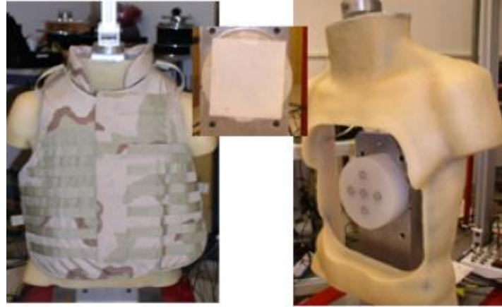
FIGURE 8-27 Left: ATM with mounted body armor. Center: ATM instrumented response element with padding. Right: oblique view of response element within torso. SOURCE: Michael Leggieri, Director, DoD Blast Injury Research Program Coordinating Office, U.S. Army Medical Research and Materiel Command, “Blunt Trauma Research to Support a New Body Armor Blunt Trauma Performance Standard and Testing Method,” presentation to the committee, August 11, 2010.
