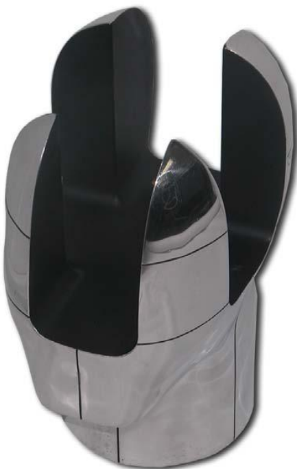
FIGURE 7-10 Army clay head form. SOURCE: Courtesy of Rob Kinsler, U.S. Army Research, Development and Engineering Command/ARL.
