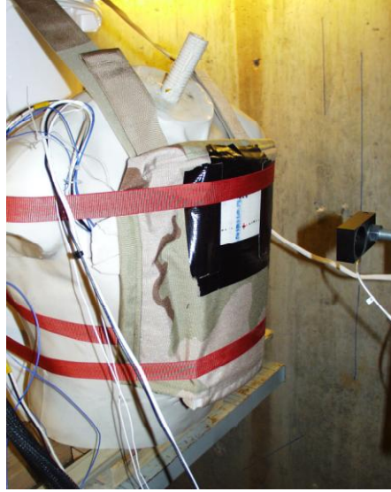
FIGURE 8-30 AUSMAN thorax with body armor in place, prior to testing. SOURCE: Reprinted with permission of Cameron Bass.
