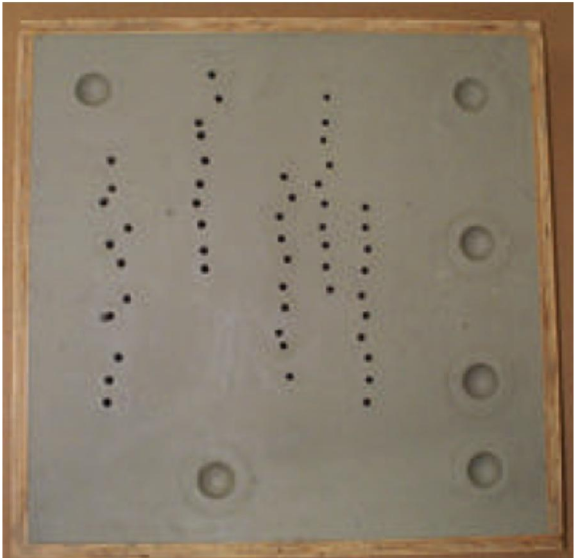
FIGURE 4-8 A clay box used for .32-cal rubber sting ball testing. The large diameter impressions represent NIJ standard calibration drops. SOURCE: Weber, 2000.
