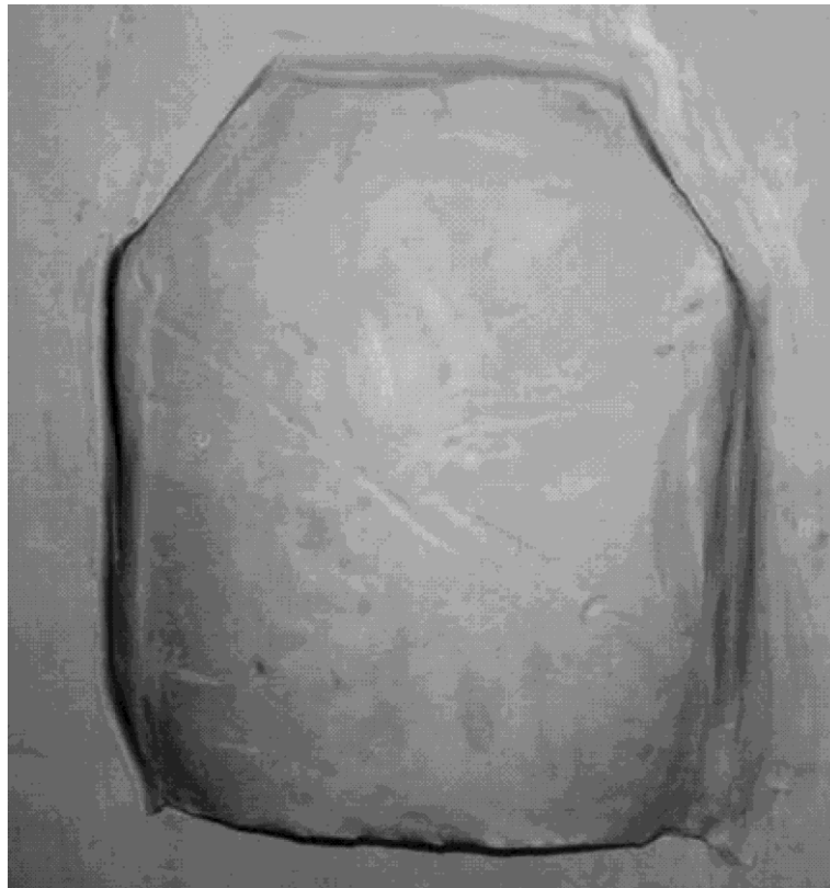
FIGURE 2-1 The clay appliqué applied to the clay box. SOURCE: Richard Sayre, Deputy Director, Office of the Secretary of Defense, Director of Operational Test and Evaluation (OSD DOT&E) Live Fire Test and Evaluation, and Tracy Sheppard, Executive Officer and Staff Specialist, OSD DOT&E Live Fire Test and Evaluation, “DoD In-Brief to the National Research Council Study Team,” presentation to the Body Armor Testing Phase I committee, Aberdeen, Maryland, November 30, 2009.
