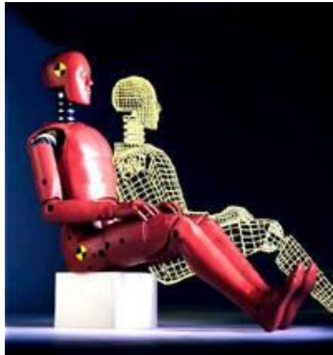
FIGURE 8-26 Hybrid III 50th percentile male dummy. SOURCE: Courtesy Humanetics Innovative Solutions.
