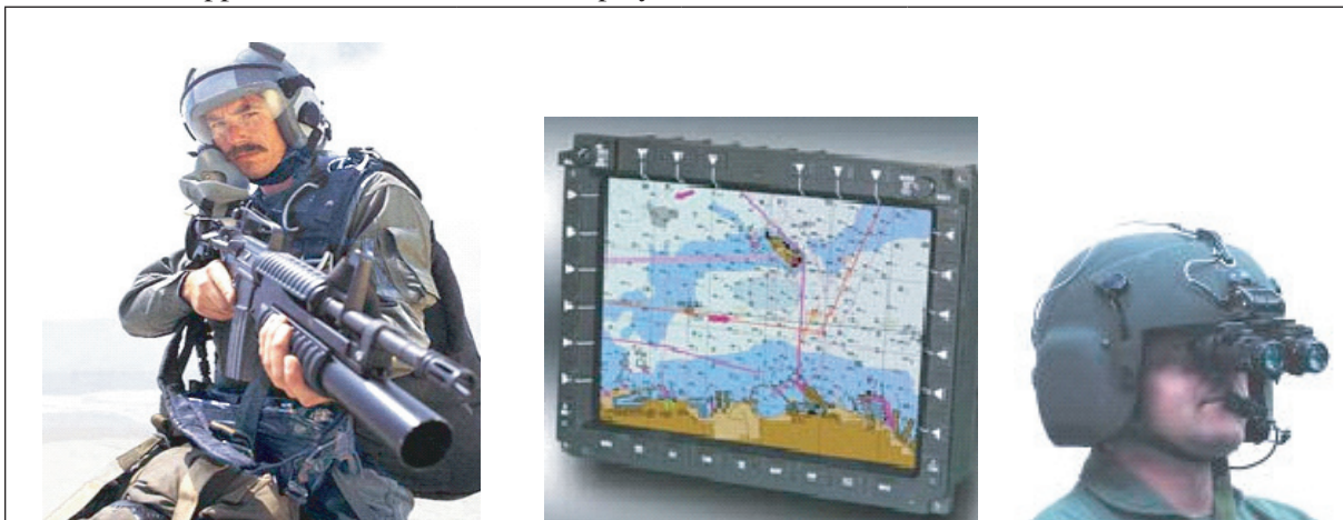
FIGURE 4-4-1 Examples of emissive displays. SOURCE: (left and right) Images courtesy of the U.S. Army; (middle) L-3 Communications (2007). Reprinted with permission.
