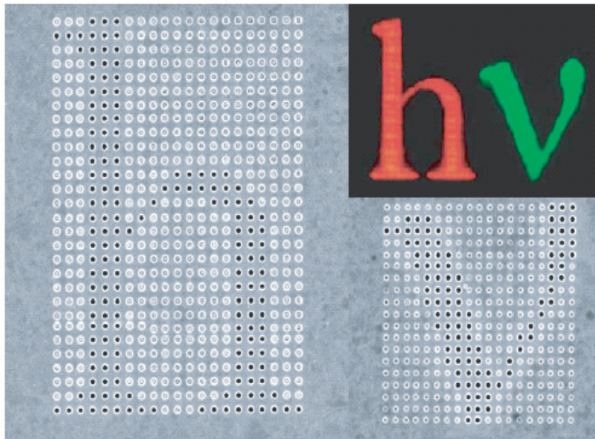
FIGURE 2-13 Scanning electron micrograph of two regions of small dimples in a silver film arranged in square arrays. SOURCE: Reprinted by permission from Genet and Ebbesen (2007). Copyright 2007 by Macmillan Publishers Ltd.
