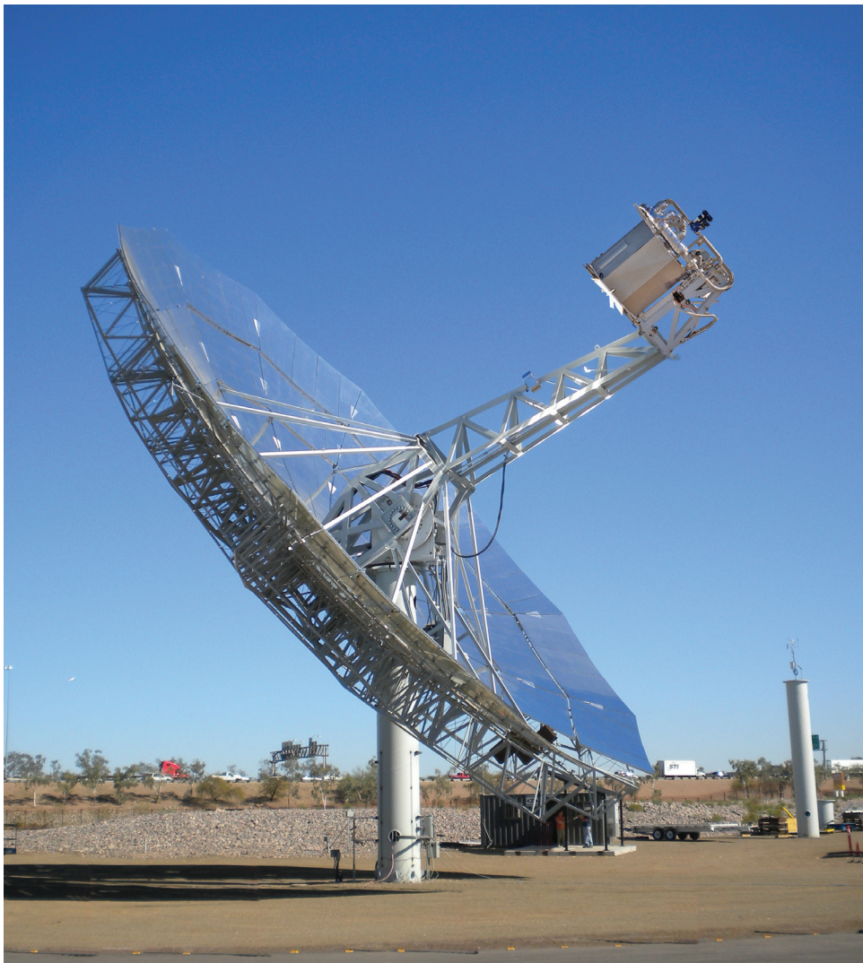
FIGURE 5.12 A dish solar thermal power generation module test unit in Phoenix, Arizona. The dish is approximately 75 feet in diameter. SOURCE: Courtesy of Southwest Solar Technologies.
