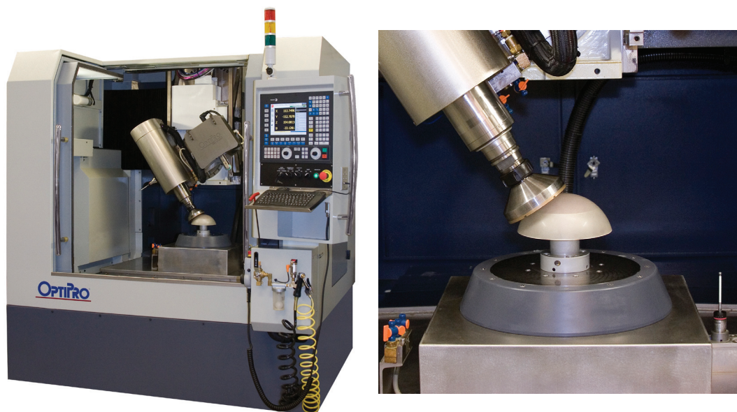
FIGURE C.8 (Left) A commercially available 5-axis computer numerically controlled grinder. (Right) A closeup image of the grinding head. SOURCE: Courtesy of Optipro.
