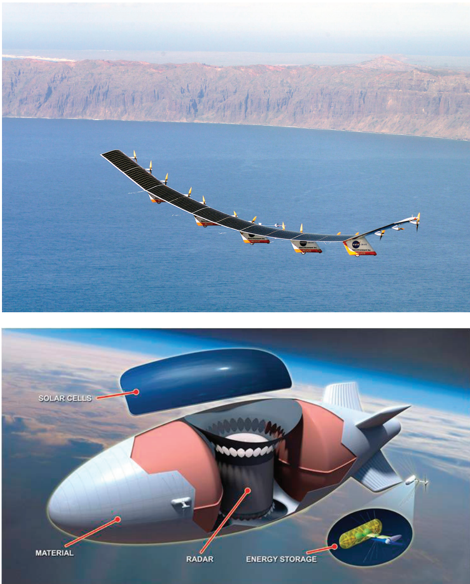
FIGURE 4.5 Overview of long-dwell platforms. (Top) The NASA Helios prototype during its test-flight over the Pacific Ocean. SOURCE: Defense Industry Daily . 2010. "DARPA's Vulture: What Goes Up, Needn't Come Down." Available at http://www.defenseindustrydaily.com/DARPAs-Vulture-What-Goes-Up-Neednt-Come-Down-04852/ . (Bottom) A depiction of the DARPA Integrated Sensor Is the Structure (ISIS) concept. SOURCE: Defense Industry Daily . 2011. "USA's HAA & ISIS Projects Seek Slow, Soaring Surveillance Superiority." Available at http://www.defenseindustrydaily.com/darpas-isis-project-seeks-slow-soaring-surveillance-superiority-updated-02189/ .
